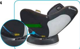
2. Remove ISOGO latches from storage slots under car seat fabrics.
