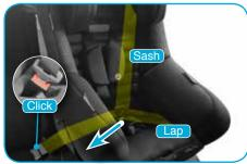
4. Thread the vehicle seat belt through the back of the seat through the YELLOW forward-facing belt path.
