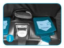
9. Pull the ISO-FIX latches out from their storage and feed them back through the fabric slots on either side of the seat so the strap is internal of the fabrics.
